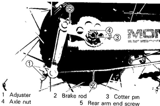
5. Push the wheel forward and remove the drive chain.
