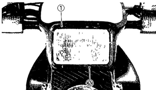
1 Horizontal adjusting screw    2 Vertical adjusting screw
