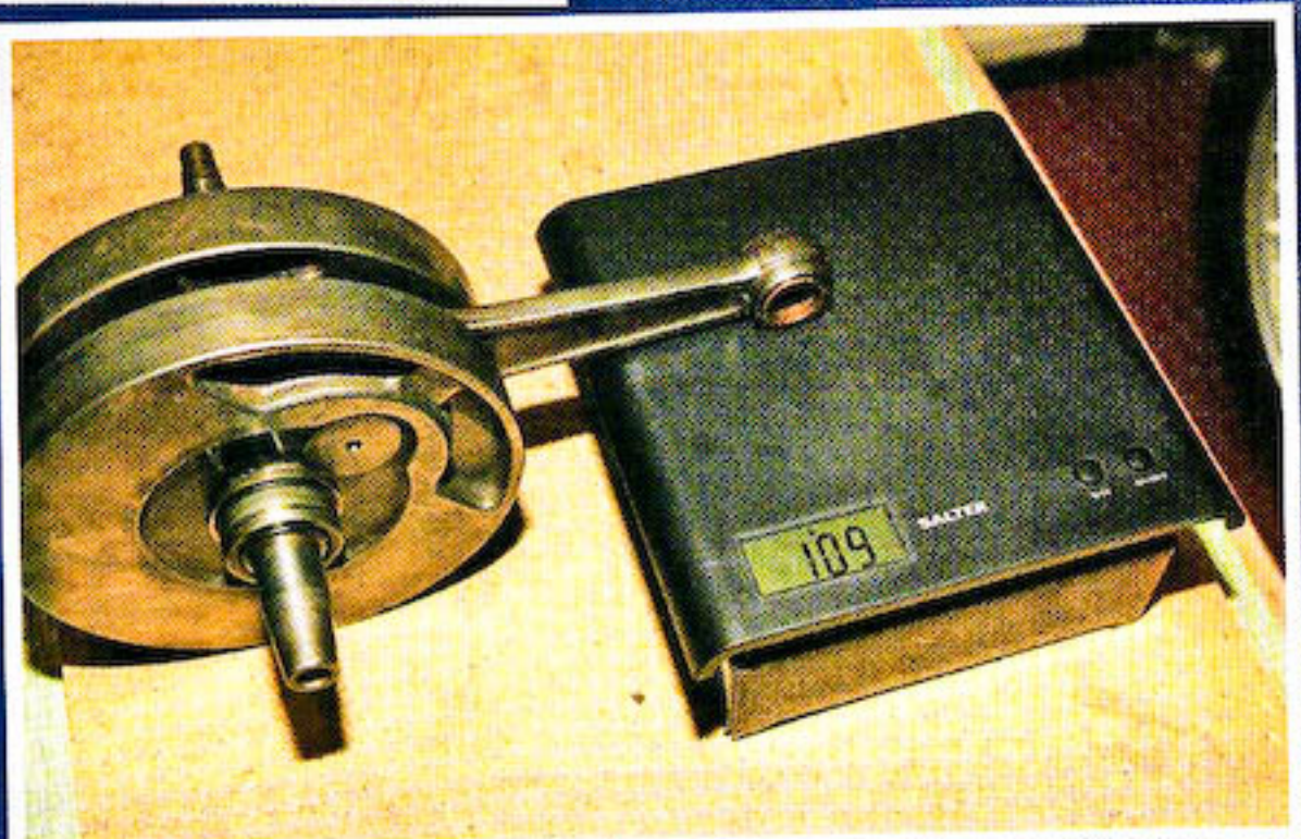
Position scales at a height to ensure upper half of conrod is weighed when at exact right angles to crankpin. Combine all reciprocating weight in this case and calculate balance factor. So 320 + 109 = 429gms include balance factor eg 66 per cent = 283gms.
