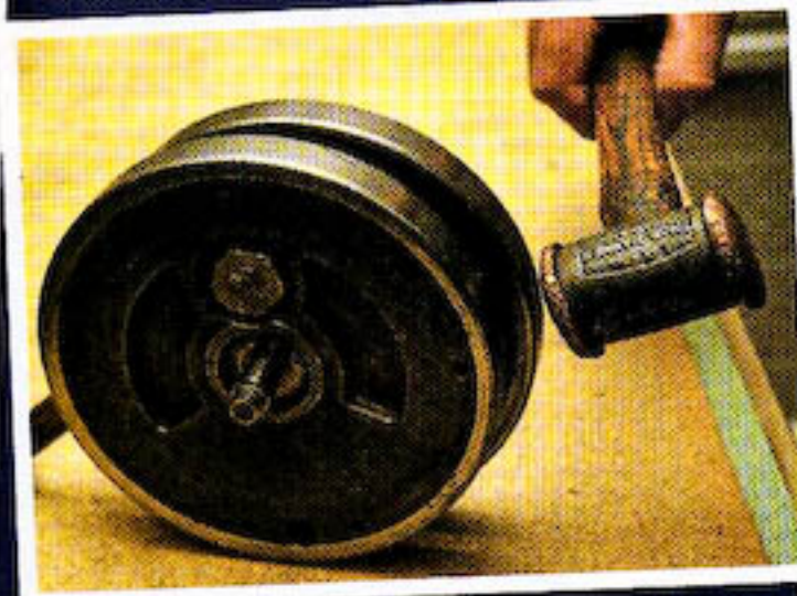
Bumping is effected by striking the rim of the errant flywheel with a copper hammer in a position at approximate right angles to the crankpin. Choice of crankshaft support while carrying out work is yours but of course such brutal work must not be carried out on the static balance knife-edge jig.
